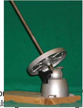
Use our No. 330 Positioner for full forms. The No. 330 is also used with partially finished shades whether built on sectional or full forms. Once the vase cap is installed put your lamp on the No. 330 and position the shade to have a level surface for final soldering.
