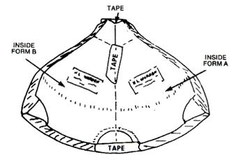
Step (4) Tack solder at least two rows of foiled glass pieces from top to bottom. DO NOT SOLDER GLASS SECTIONS TOGETHER. Bridging pieces will extend from one form to the other. If the glass sections are soldered together by mistake....remelt and separate.
