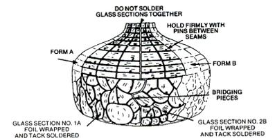
Step (6) Repeat steps 3, 4 and 5, only labeling the glass section on the left 2B. As each glass section is made by alternating the forms; label the next sections 3A, 4B and 5A. The sections will look the same, but for instance, section 3A fits ONLY to the left of 4B and at the same time fits ONLY to the right of 2B.
