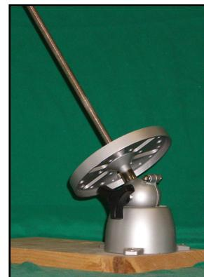
Use our No. 330 Positioner for working with full forms. The No. 330 is also great for working with partially finished shades whether built on sectional or full forms. Once the vase cap is installed put your lamp on the No. 330 and position the shade to have a level surface for final soldering.
