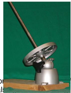
Use our No. 330 Positioner on full forms. The No. 330 is also used with partially finished shades whether built on sectional or full forms. Once the vase cap is installed put your lamp on the No. 330 and position the shade to have a level surface for final soldering.
