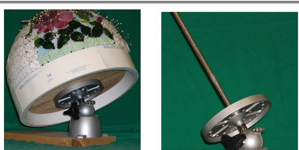
Use our No. 330 Positioner for full forms. The No. 330 is also used with partially finished shades whether built on sectional or full forms. Once the vase cap is installed put your lamp on the No. 330 and position the shade to have a level surface for final soldering.
