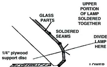
(6) DO NOT BUILD ROUNDED SEAMS ON THE FORM. Remove the lamp and fill and then build the inside seams then do the outside. By filling the inside first, any flow through will be removed when building the outside seams.
