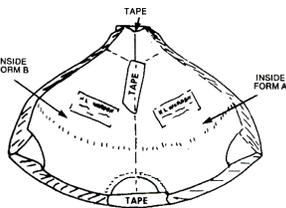
Step (3) With the two forms fastened together; cut, grind, foil and pin glass pieces on both forms including the bridging
