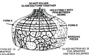
MUST BE MOVED TO THE LEFT TO FIT THE GLASS PIECES ON THAT SIDE TO THE OTHER GLASS SECTION.
