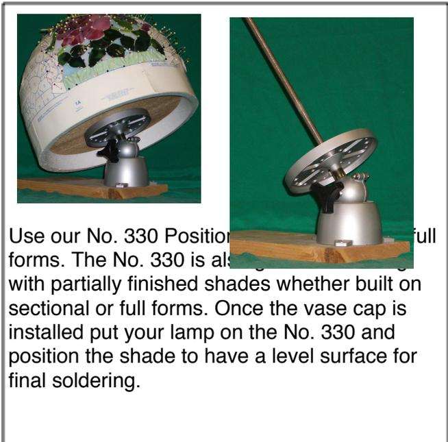
Use our No. 330 Positioner forms. The No. 330 is also used with partially finished shades whether built on sectional or full forms. Once the vase cap is installed put your lamp on the No. 330 and position the shade to have a level surface for final soldering.
