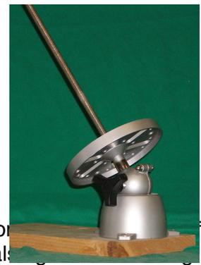
Use our No. 330 Positioner for full forms. The No. 330 is also used with partially finished shades whether built on sectional or full forms. Once the vase cap is installed put your lamp on the No. 330 and position the shade to have a level surface for final soldering.
